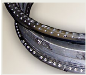
Detail of Intermediate Pressure Casing – the vertical and horizontal operations can be done by using the main spindle and right angular head
