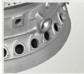
Detail of combustor structure – the angled features are machine by using the 5-axes positing capability of the nutating head in the Unicom 6000-HV machining centre
