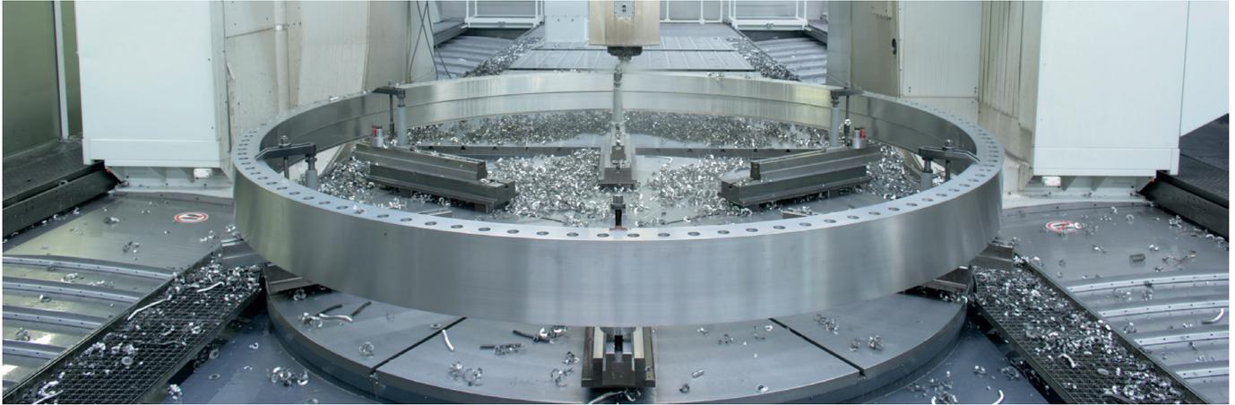
large component. Here at Brück, a component weighing 3 tonnes is classed as a small component. To give just one example: Wind turbines contain large rings that control the power transmission system. Rings of that type are the sort of products we typically produce.”
