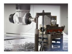
the increased availability that is provided by two identical machines. The large tool magazine also offers several key advantages. Dohnalek said: "In each machine, we have 197 tool places. Normally, machines have only 27 places as standard. Unisign increased the number of tool places especially for us. As we machine a variety of materials, we also need a variety of tooling."
