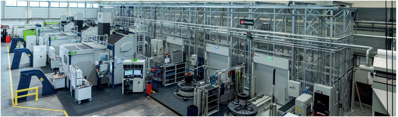
to a higher level, we decided to implement a total solution concept by linking three UNICOM6000 machines to a pallet-handling and warehousing system – a Fastems Flexible Manufacturing System (FMS). Of all suppliers we considered, Unisign was the one that came up with the most effective total solution.” A one-off contract was issued for the solution as a whole (3x UNICOM with an FMS), and the lead role was entrusted to Unisign.
