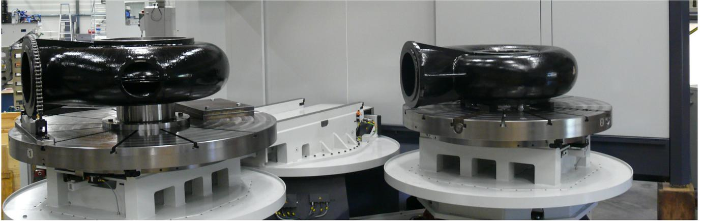
we produce have a diameter of around 1.3 metres and are over 2000 mm high. The components that we drill, turn and mill using our UNICOM6000 always consist of 1 to 3 individual pieces per set, in a variety of sizes. In most cases, they are made of cast iron.”
