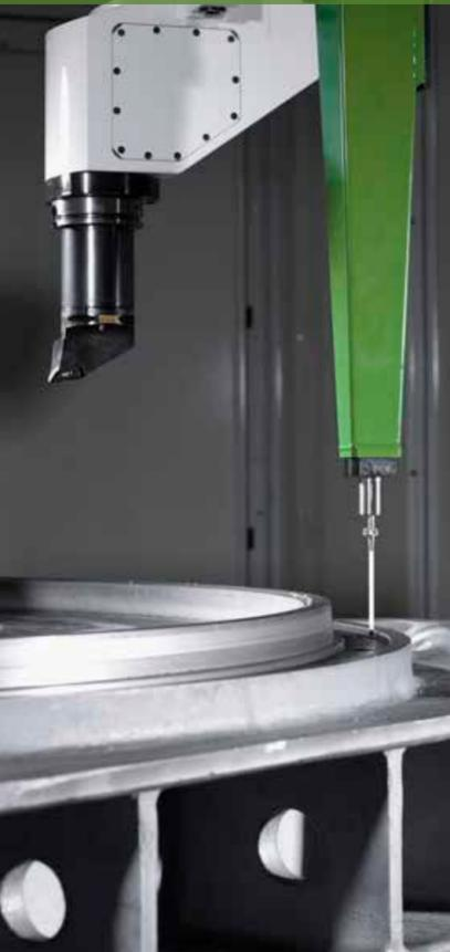
In-process measuring probe
