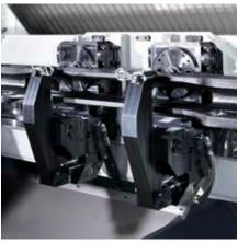
One further strong point of the UNISIGN front axle machining solutions is their flexibility. With minimum effort, the fixture can be altered to allow a large variety of front axles to be clamped. There is even an option to change the full fixture, which allows customers to produce less common types of beams, such as bus front axles.
